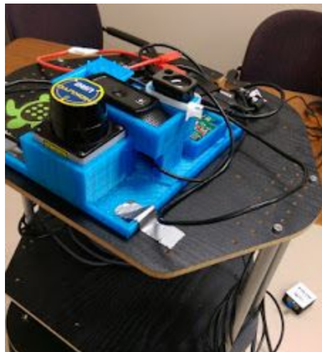
Figure 39: Casing for Sensors[6]
